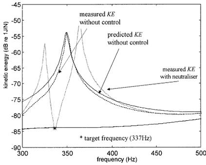
(a) Neutralizer no. 1 with  $\omega_a=335\text{Hz}$
