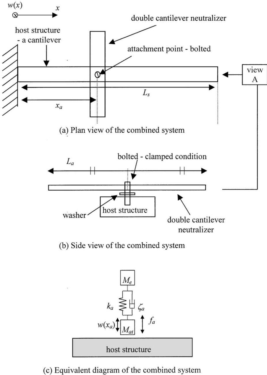
Fig. 2. Schematic diagram represent the combined system and its equivalent model.  $L_s$ ,  $x_a$ , and  $L_a$  are the length of the cantilever, the location of the neutralizer on the cantilever and the length of the double cantilevers neutralizer respectively.  $\otimes$  means the axis is pointing out of the page.
