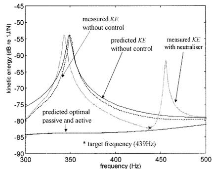
(f) Neutralizer no. 6 with  $\omega_a=446\text{Hz}$
