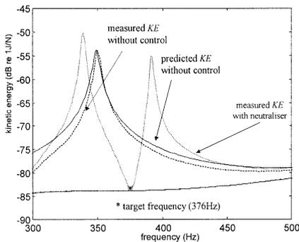
(c) Neutralizer no. 3 with  $\omega_a=376\text{Hz}$
