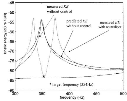
(b) Neutralizer no. 2 with  $\omega_a=353\text{Hz}$
