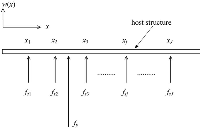
Fig. 1. An arbitrary structure with control devices attached.  $f_p$  is the primary force,  $f_{s1}, f_{s2}, \dots, f_{sJ}$  are the secondary forces, and  $x_{s1}, x_{s2}, \dots, x_{sJ}$  are the location of the forces on the host structure.
