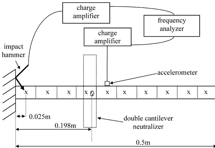
Fig. 3. Experimental set-up to determine the effect of the application of an optimally detuned neutralizer to the kinetic energy of the cantilever. X—location of the accelerometer.
