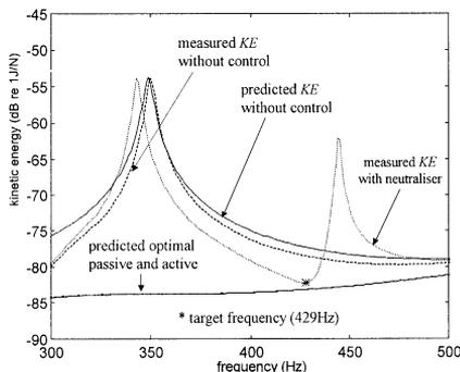
(e) Neutralizer no. 5 with  $\omega_a=434\text{Hz}$
