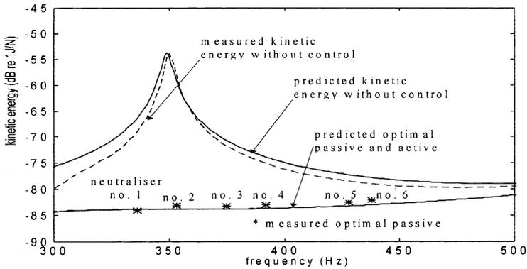
Fig. 5. Experimental results on the kinetic energy of the cantilever using neutralizer with optimal tuning ratio at the targeted frequencies. The \*s are the measured kinetic energy at the target frequencies of the neutralizer with the optimal frequency attached.  $M_e$  for predicted optimal passive is fixed at 0.0082 kg and the result from active control is used as a benchmark.
