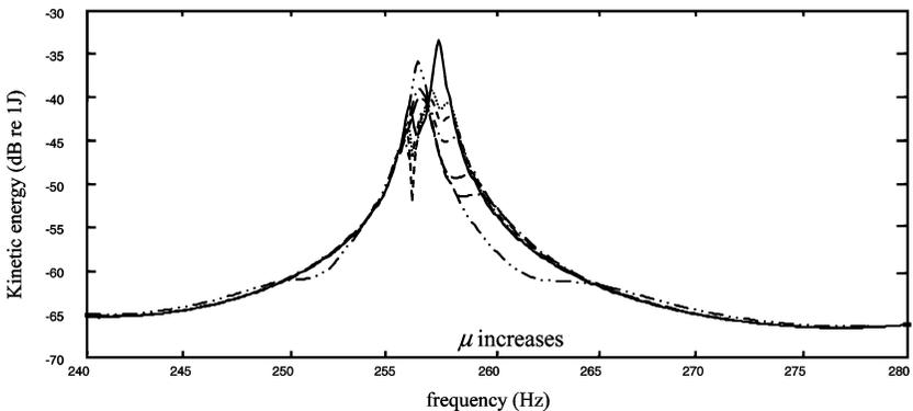
**Figure 8.** Effects of the neutralizer that was optimized to the eleventh natural frequency on the kinetic energy of the plate. The neutralizer is applied at  $(0.375L_x, 0.25L_y)$  and  $\mu = 0.0005, 0.00005, 0.00003, 0.00001, 0.000005,$  and  $0.000003$ .
