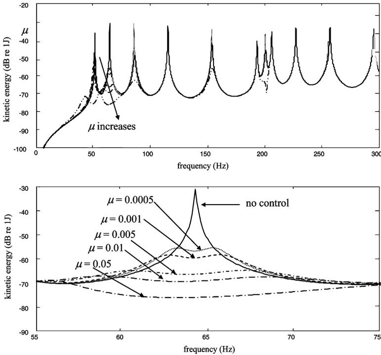
**Figure 2.** Effects of the optimal vibration neutralizer on the kinetic energy of the plate where the neutralizer is optimized to the second natural frequency and is applied at  $(0.25L_x, 0.5L_y)$ . (a) Overall kinetic energy and (b) kinetic energy in the vicinity of the second natural frequency.
