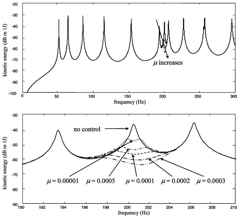
**Figure 5.** Effects of the neutralizer that was optimized to the seventh natural frequency on the kinetic energy of the plate. The neutralizer is applied at  $(5L_x/12, 0.5L_y)$ . (a) Overall kinetic energy and (b) kinetic energy in the vicinity of the seventh natural frequency.
