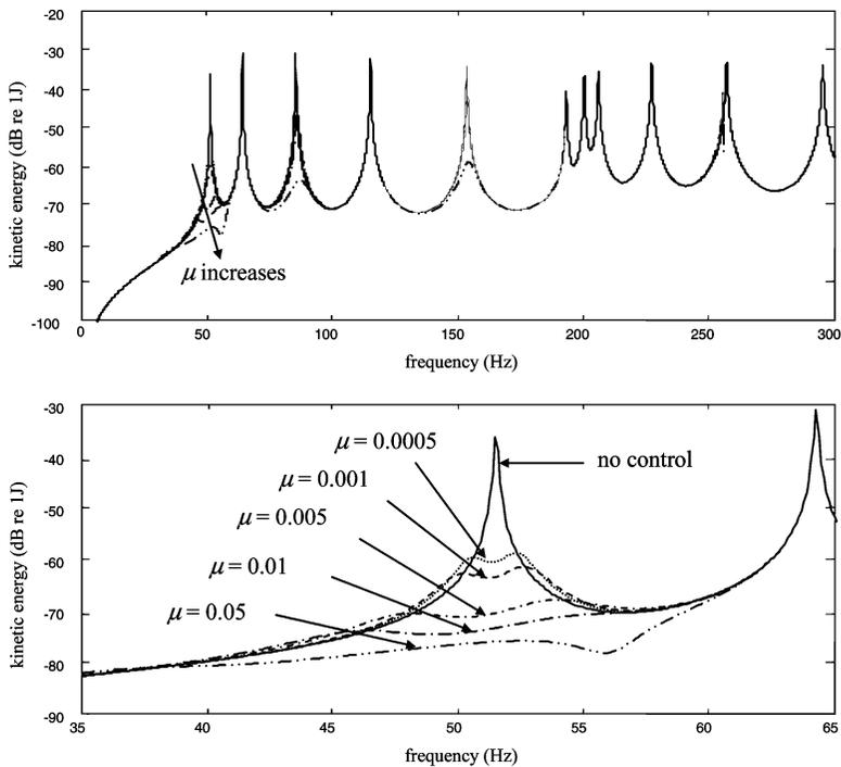
**Figure 1.** Effects of the optimal vibration neutralizer on the kinetic energy of the plate. The neutralizer is optimized to the first natural frequency and is applied at  $(0.5L_x, 0.5L_y)$ . (a) Overall kinetic energy and (b) kinetic energy in the vicinity of the first natural frequency.
