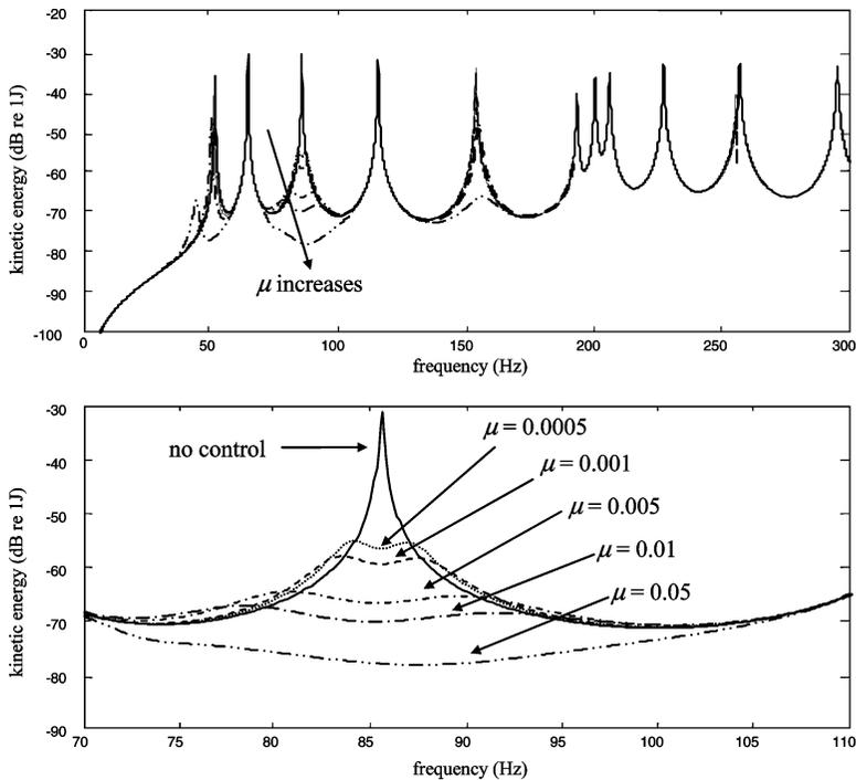
**Figure 3.** Kinetic energy of the plate with neutralizer optimized to its third natural frequency and is applied at  $(0.5L_x, 0.5L_y)$ . (a) Overall kinetic energy and (b) kinetic energy in the vicinity of the third natural frequency.
