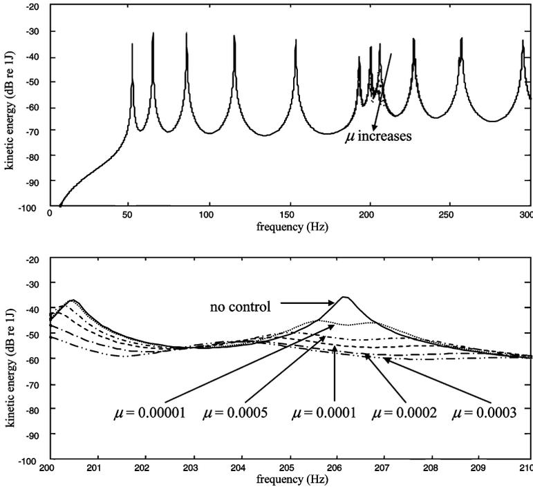
**Figure 6.** Effect of the neutralizer that was optimized to the eight, natural frequency on the kinetic energy of the plate. The neutralizer is applied at  $(0.25L_x, 0.25L_y)$ . (a) Overall kinetic energy and (b) kinetic energy in the vicinity of the eighth natural frequency.
