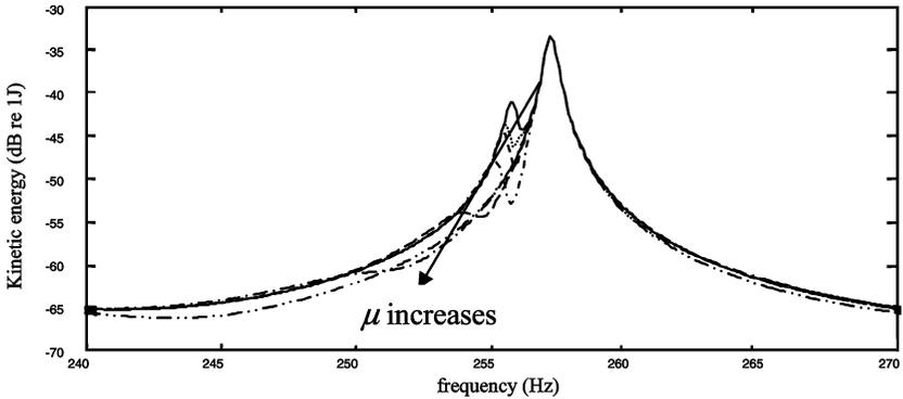
**Figure 7.** Effects of the neutralizer that was optimized to the tenth natural frequency on the kinetic energy of the plate. The neutralizer is applied at  $(0.25L_x, 0.25L_y)$  and  $\mu = 0.005, 0.0005, 0.00005, 0.000005, 0.0000005,$  and  $0.0000001$ .
