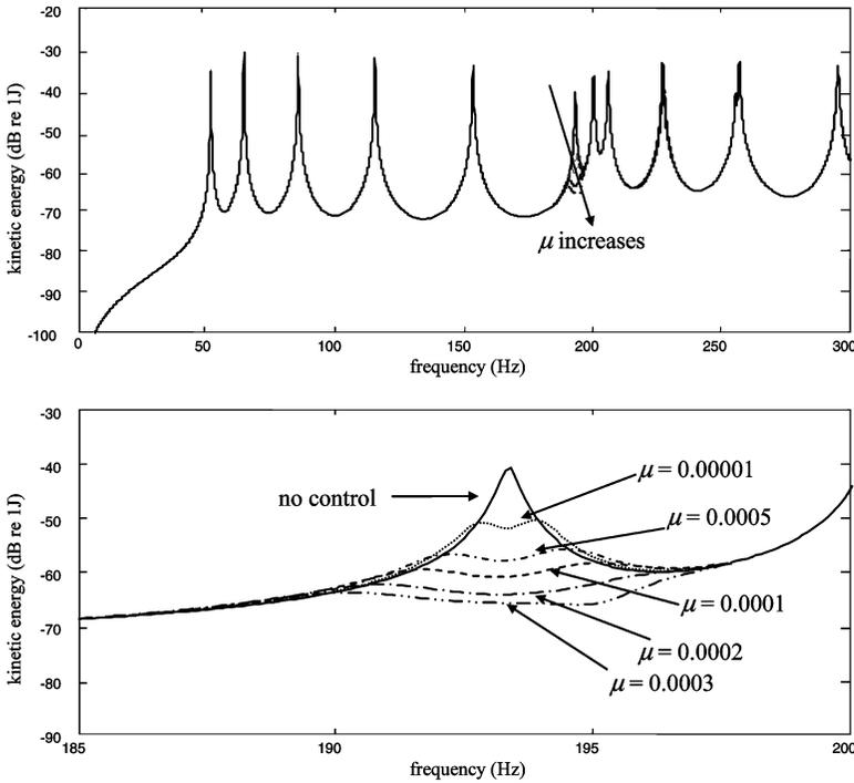
**Figure 4.** Effects of the neutralizer that was optimized to the sixth natural frequency on the kinetic energy of the plate. The neutralizer is applied at  $(0.5L_x, 0.25L_y)$ . (a) Overall kinetic energy and (b) kinetic energy in the vicinity of the sixth natural frequency.
