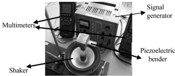
Fig. 5 Setup of the experiment with the single piezo composite bender
