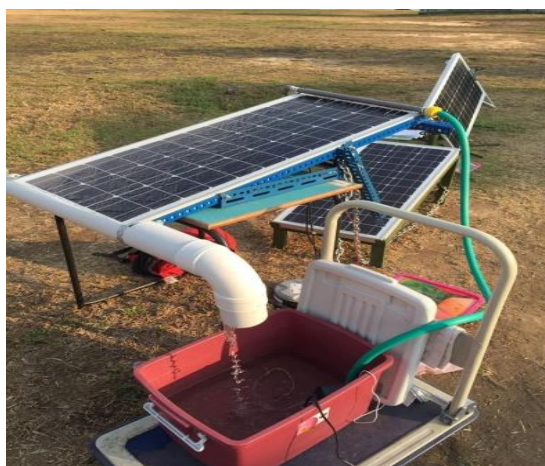
Fig. 1. Experimental setup of cooling system.
