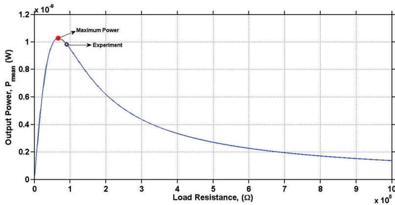
Figure 10. Mean output power versus different load resistances in a certain frequency (228 rad/s).
