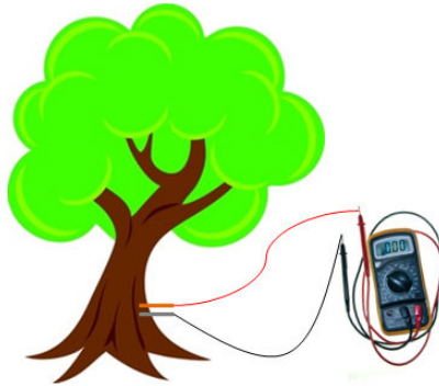
Figure 1: Connection between the electrode pairs to the trees and the multi-meter.
