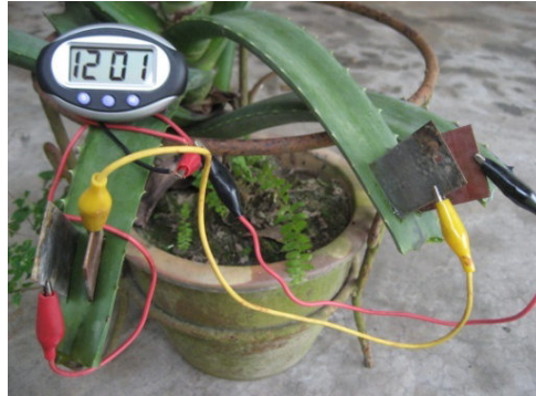
Figure 7: A digital clock powered by organic energy source
