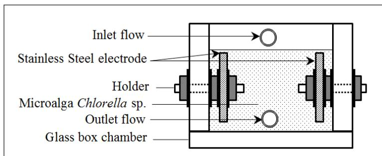
Figure 1. Schematic diagram of the ET chamber (front view)
