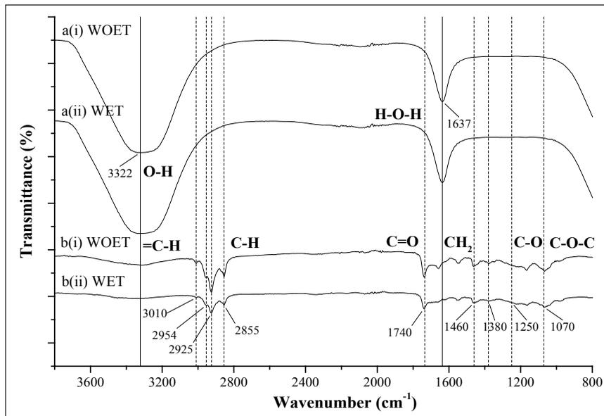
Figure 2. (a) FTIR spectra of (i) *Chlorella* sp. D<sub>WOET</sub> and (ii) *Chlorella* sp. D<sub>WET</sub> prior to solvent extraction. (b) FTIR spectra from (i) *Chlorella* sp. D<sub>WOET</sub> and (ii) *Chlorella* sp. D<sub>WET</sub> after solvent extraction
