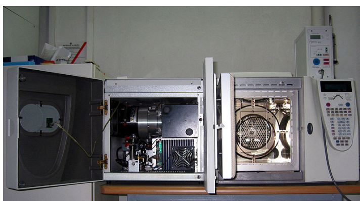
The insides of the GC-MS, with the column of the gas chromatograph in the oven on the right.
