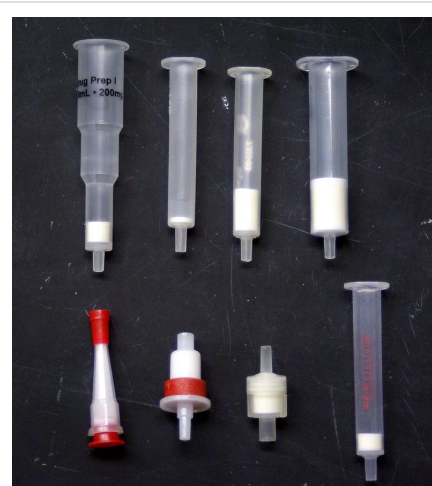
A selection of solid phase extraction cartridges, available in many sizes, shapes, and types of stationary phase.
